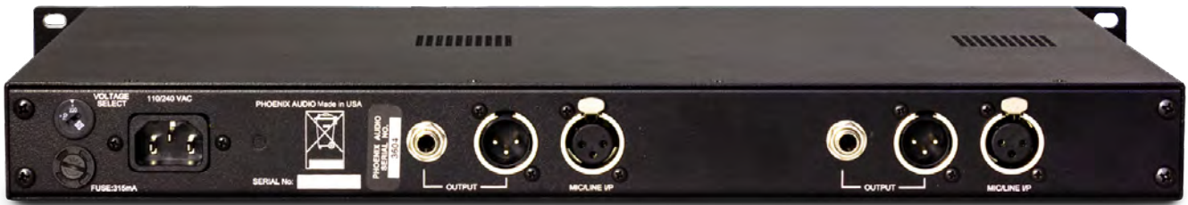
The balanced analogue outputs are presented on both XLR and TRS jack sockets.
