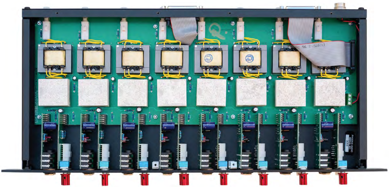
With all the Class-A circuitry and output transformers, there really is no room to spare for a built-in power supply!
