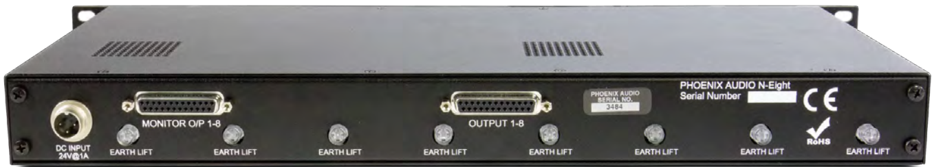
Both the main and monitor outputs are delivered via D-sub. Although each output is tapped from a different side of the same transformer, the design means that they always sound identical, differing only in level.
